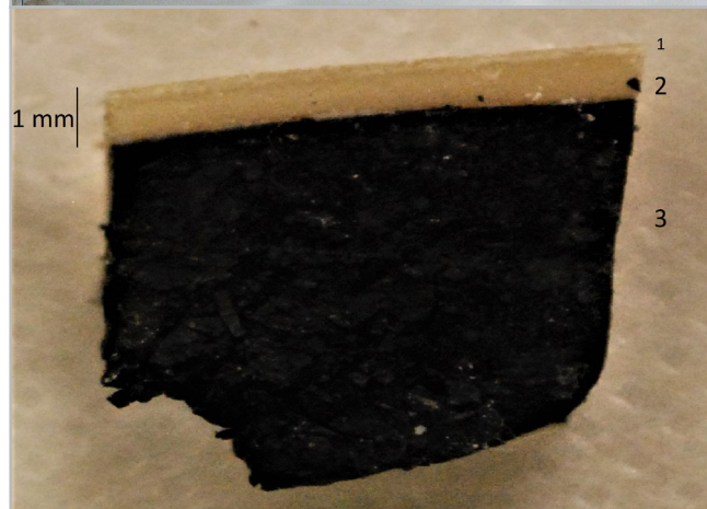
Figure 8.- At the top: micrograph of crystals. The lower part shows a stratigraphy of a clean sole area. For this reason, no whitish residue is visible. The image stands out because it shows the perfect adhesive bond between the polyurethane and the Phylon. With number one, a thinner, lighter layer is also visible where the degradation of the polyurethane begins. Next, with number two, a darker layer of polyurethane in a better state of conservation, and with number three, the Phylon in perfect condition. Photograph: own authorship.
