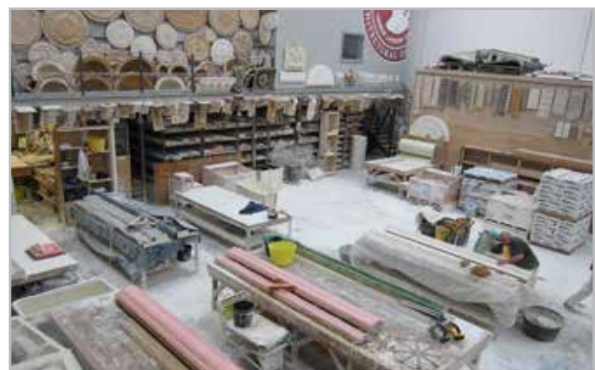
Figure 6.- London George Jackson Limited. General view of the workplace and storage of the wooden contra moulds. Jackson & Sons produced wooden contra malls by specialists woodcarvers. A complicated tecnique because of the three-dimensional thinking in reflection. ©W. Freling.
