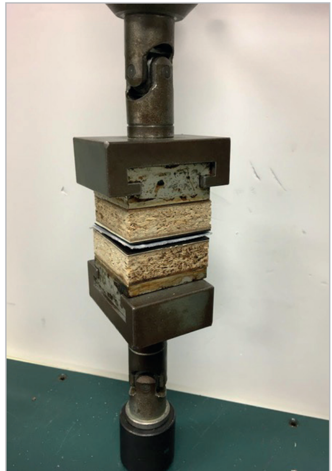
Figure 1.- Tensile strength test results with various magnetic sheets and supports.
